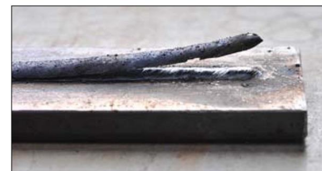
Fig.4: Convenient self-peeling slag removal with RB-26 assures a glossy bead appearance without post-weld brushing
